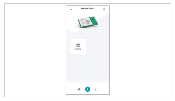
The default software running on the PAN9026-IMX provides access to the Wi-Fi and Bluetooth features of the PAN9026 module by supplying a web server running on a Wi-Fi access point. After a connection to that access point is established, it is possible to interact with the PAN9026 module (with the browser).
