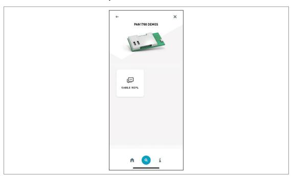
In the demo "Cable Replacement", the module acts as a Bluetooth LE peripheral device and emulates a remote device that exchanges data with the mobile device.
